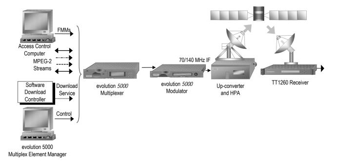
Figure 1.5: Typical Download Transmission System
